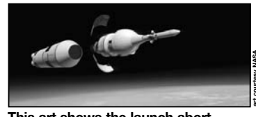
This art shows the launch abort system (far right) still attached.
