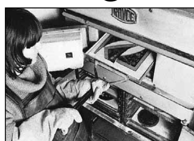
Next, the painted glass is fired in a kiln, a super-hot oven that fuses the paint to the glass. Then it's allowed to cool slowly.
