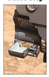
This NASA image shows the Curiosity rover with a scoop of powdered rock on Mars. The rover drilled into a Martian rock for the first time and transferred a pinch of powder to its instruments to anachemical makeup.
