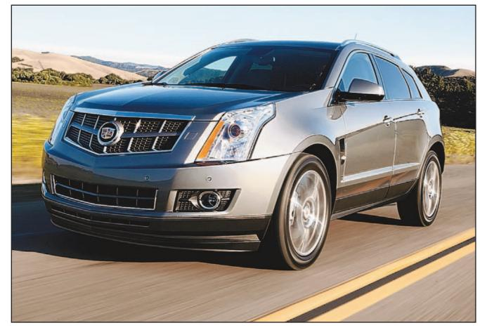
The Cadillac SRX enters 2012 with a greater combination of performance, technology and capability. A new, more powerful 3.6liter V-6 engine becomes the sole engine offered in the SRX. It's rated at 308 horsepower and 265 lb.-ft. of torque.
