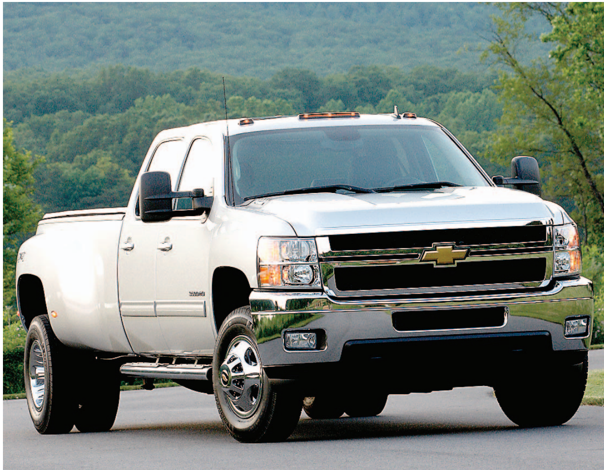
2011 Silverado and Sierra heavy-duty pickups offer increased power, and upgraded towing and payload capacity. A more-potent Duramax diesel, beefier frame, and new front and rear suspension systems highlight the improvements. The Duramax 6.6-liter turbodiesel delivers more horsepower and torque, and improved fuel efficiency (11 percent increase) and emissions (63 percent reduction).
