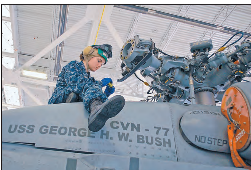
AD2 Donna Beaman inspects the main rotor in preparation for “hanging the blades” on an MH-60R Seahawk in Hangar 1122 at NAS Jax.
