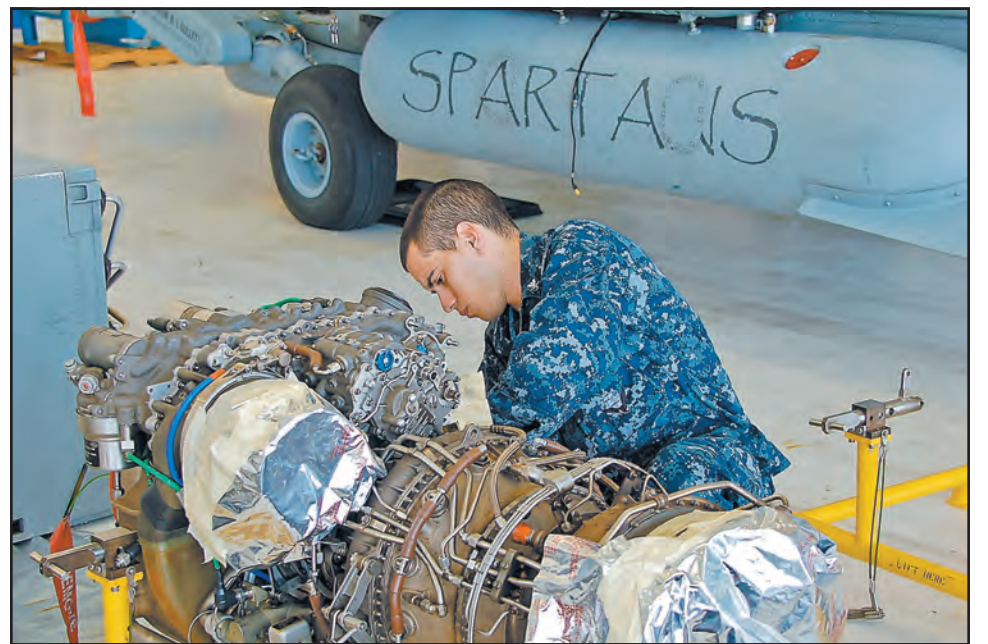
ADAN Frankie Morales prepares a T700-GE-401C turboshaft engine for installation in an MH-60R Seahawk assigned to the HSM-70 Spartans.
