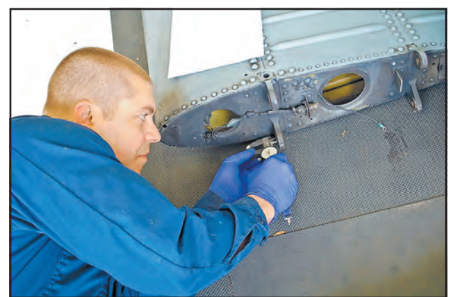
AM3 Cody Blackwell uses an inside caliper to measure a bushing in the horizontal stabilizer of an MH-60R Seahawk helicopter assigned to the Spartans of HSM-70.
