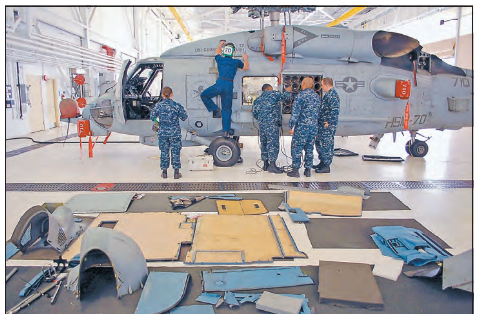
In NAS Jacksonville Hangar 1122, HSM-70 maintainers inspect the sonobuoy launcher of MH-60R Seahawk No. 710, that will also have its main rotor blades attached by end of the day.
