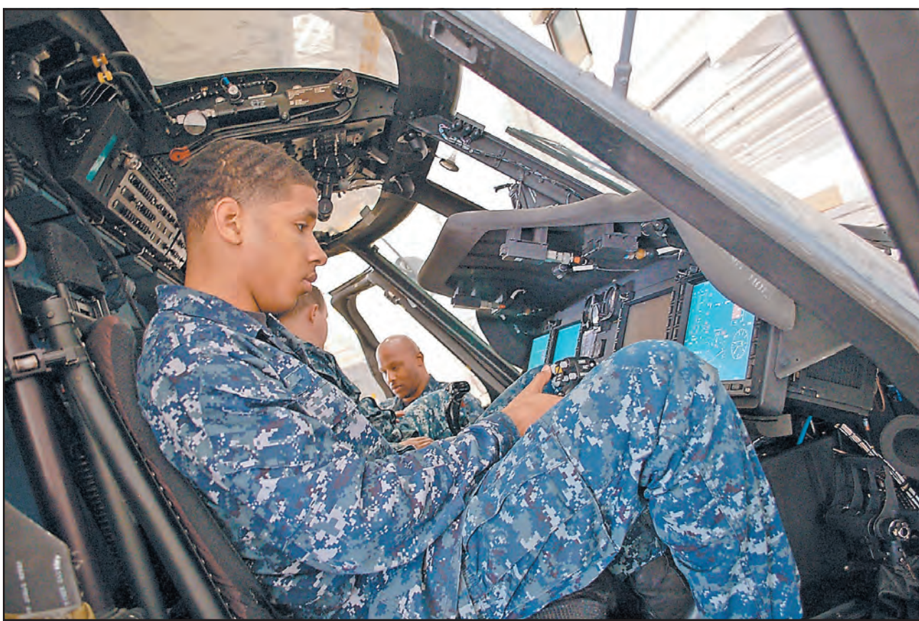
AOAN Marcus Bunk monitors the armament release and control systems test of an AGM-114 Hellfire missile.
