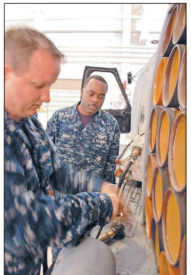
AO1 Aaron Ammons and AO2 Alpha Uzoma inspect and repair the sonobuoy launch array used for submarine detection and tracking.
