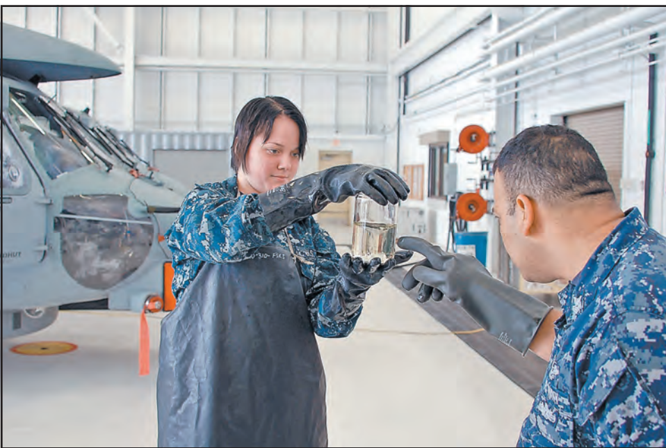
AN Melissa Mowry pulls a fuel sample from an MH-60R Seahawk helicopter for inspection by AD1 Wilfredo Briones, who declares it "clean and dry" – and ready to fly.
