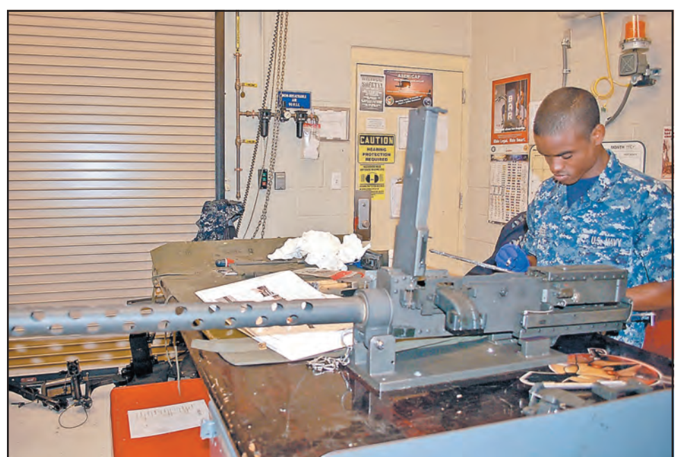
AOAN Markus James cleans and inspects a .50 caliber GAU-21 machine gun. Also known as the M3M, the GAU-21 is an updated machine gun that serves as the primary suppressive fire system for Navy and Marine Corps helicopters.
