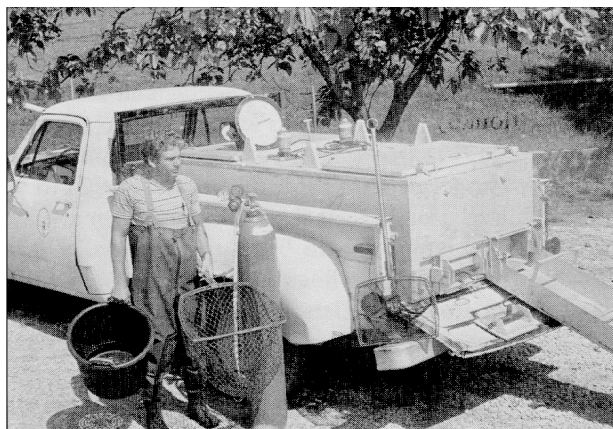
Figure 8. Tank with aerator for hauling fingerlings.
