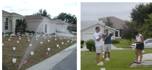
Figure 2. Irrigation uniformity bucket test Credits: Melissa B. Haley
