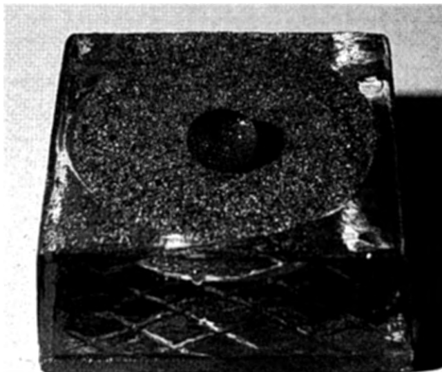
Fig. 1. Water drop on unconsolidated water repellent sand.
