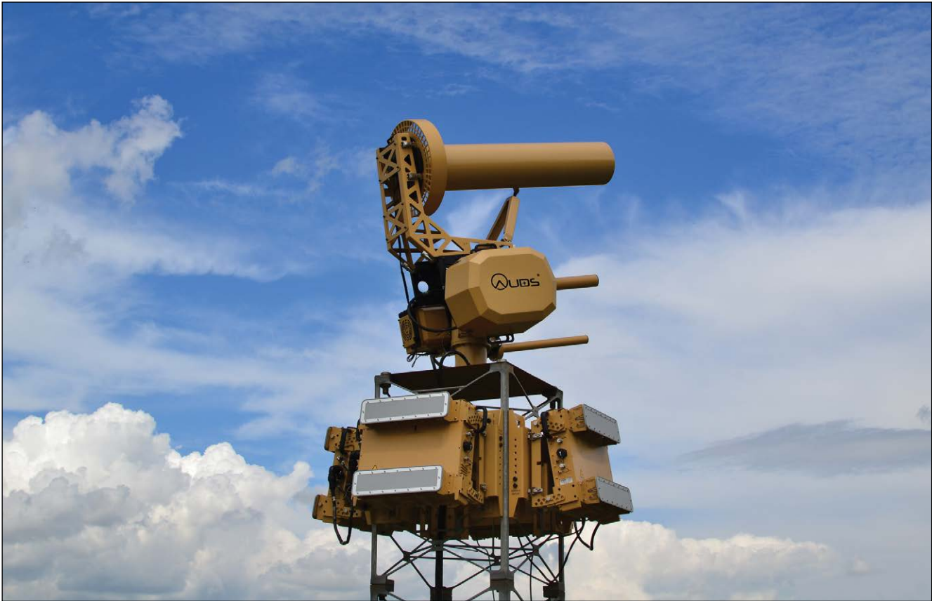
AUDS is a counter-drone system designed to disrupt and neutralize unmanned aerial vehicles.
