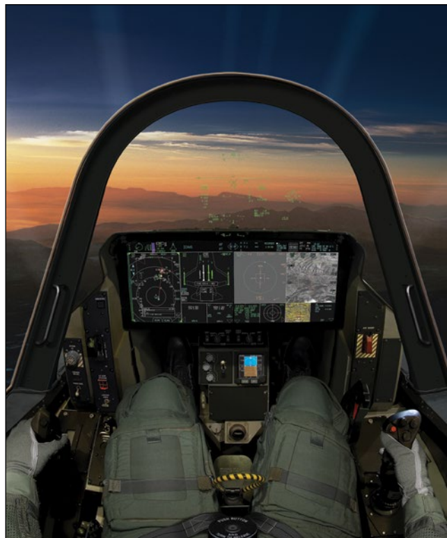
The high-technology large area display glass cockpit of the F35A Lightning II .
