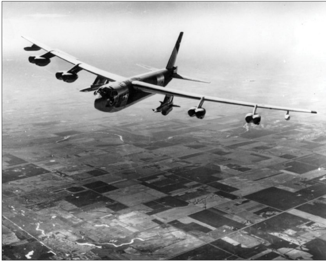
A B-52 Stratofortress with air launched Hound Dog cruise missiles under each wing
