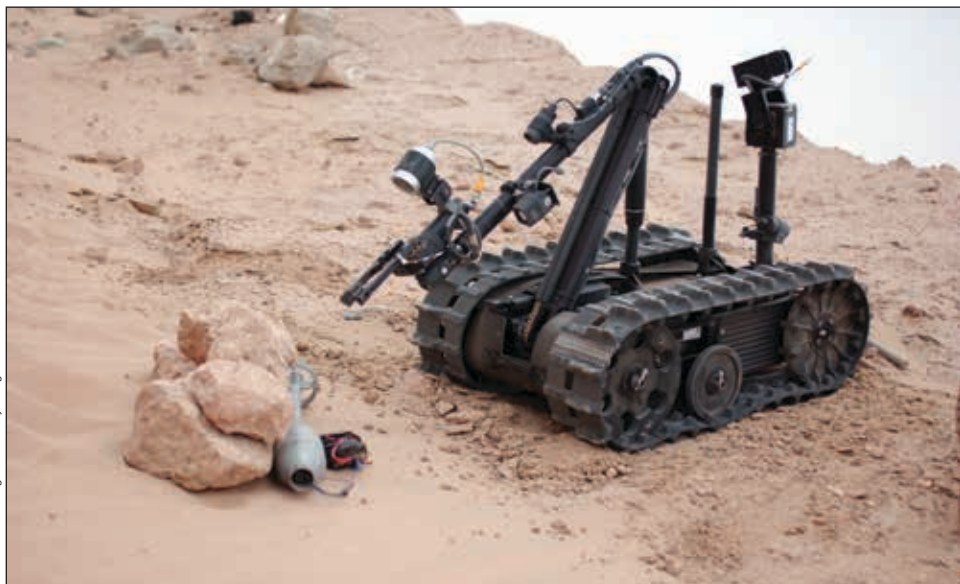
A Talon robot goes in for a closer look at a suspected improvised explosive device.
