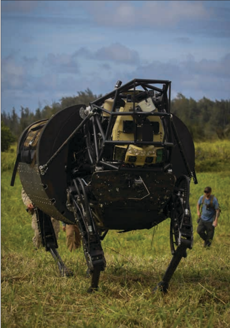
The Legged Squad Support System Big Dog , a load-carrying robotic quadruped being tested during Exercise RIMPAC.
