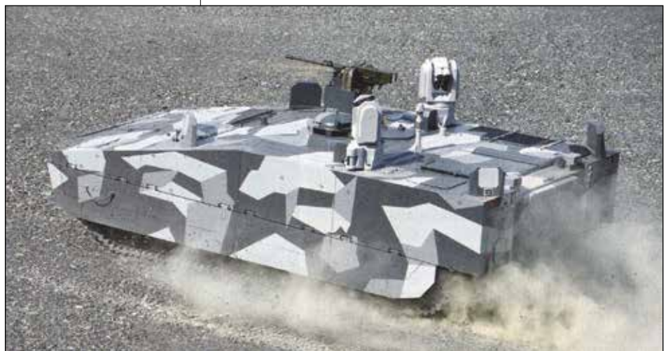
Saab LEDS 150 fitted to a BAE Systems CV 90 Armadillo .
