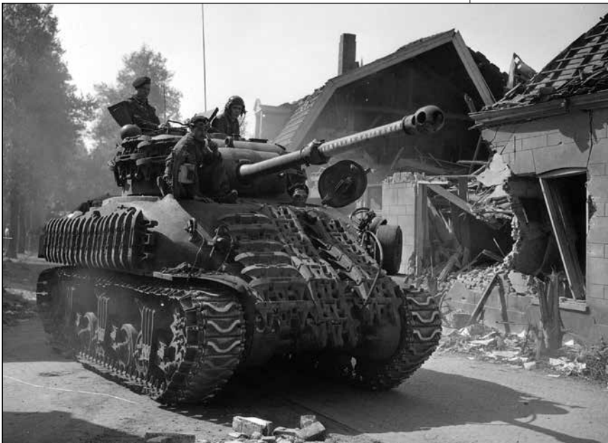
A Canadian 8 th Hussars Firefly tank passes through Putten in Holland on the way to the Zuider Zee, 18 April 1945. Note the different varieties of steel track welded to the front of the hull for additional protection.
