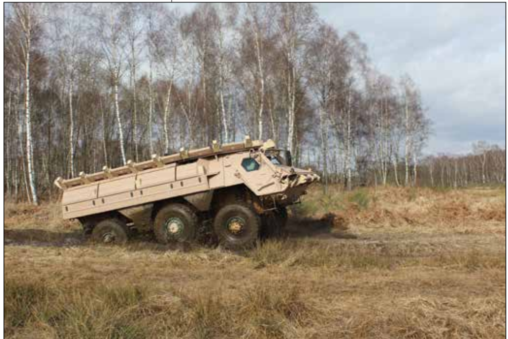
A RMMV Fuchs 1 A8 IFV equipped with ADS HAT ~ A full rocket and missile Active Defence System.
