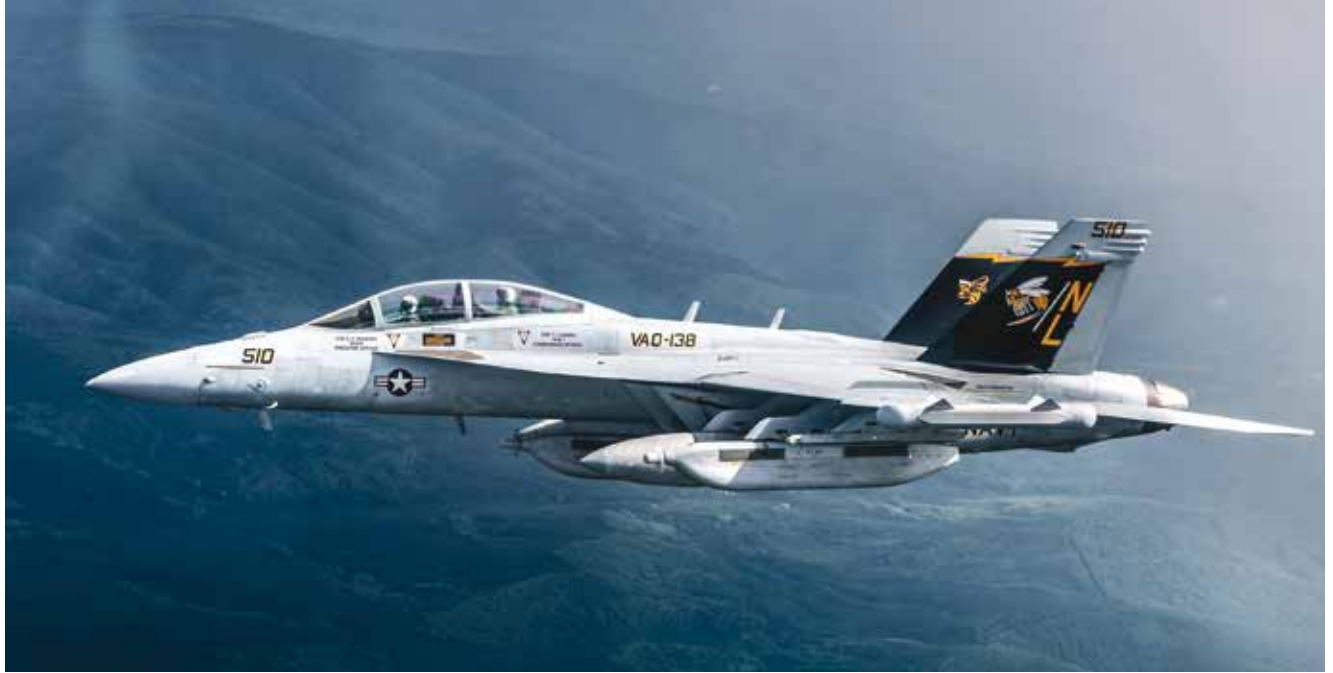
The EA-18G Growler is the world's only tactical electronic attack aircraft. Growlers can locate and jam enemy ships, aircraft, radars and communications, as well as fire air-to-surface and air-to-air missiles.
