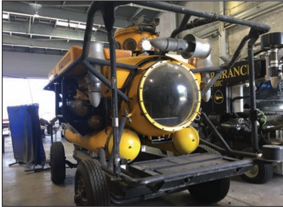
One of the historic Johnson Sea Link submersibles (now retired) on display at FAU – Harbor Branch Oceanographic Institute.
