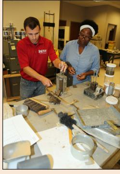
David Little, left, and Hattie Johnson, right, trim an undisturbed soil sample for an undrained triaxial test.
