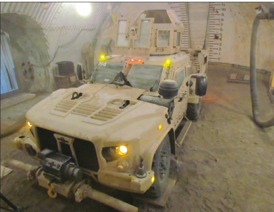
Among other things, the JLTV undergoes frosty conditioning in a cold chamber on post. The chamber itself is contained within a transition environment that buffers test personnel rooms from the extreme temperatures inside, and is outfitted with items such as cameras and air quality monitors.
