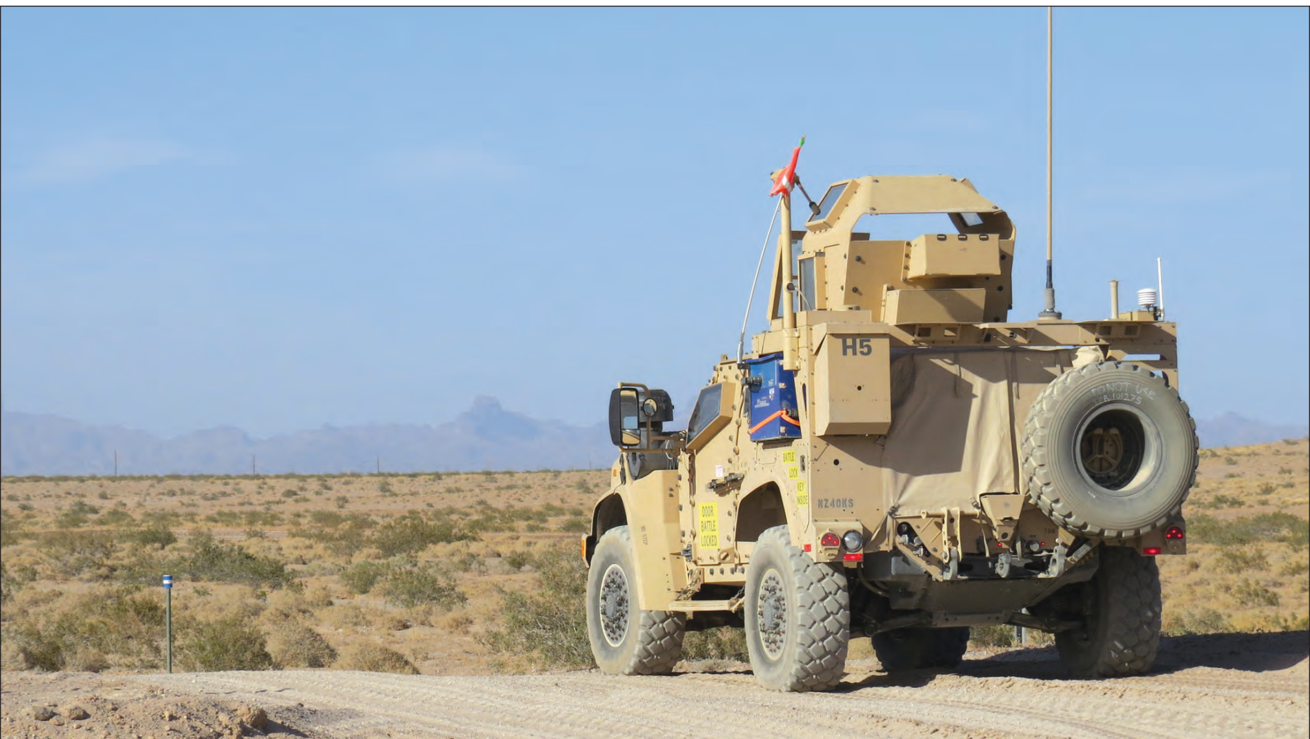
In addition to running the vehicles across 36,500 miles of paved, secondary, trails and cross-country roads at YTC, YPG testers are testing everything from the overhead gunner's protection kit to vehicle's active suspension system. (US Army photos)
