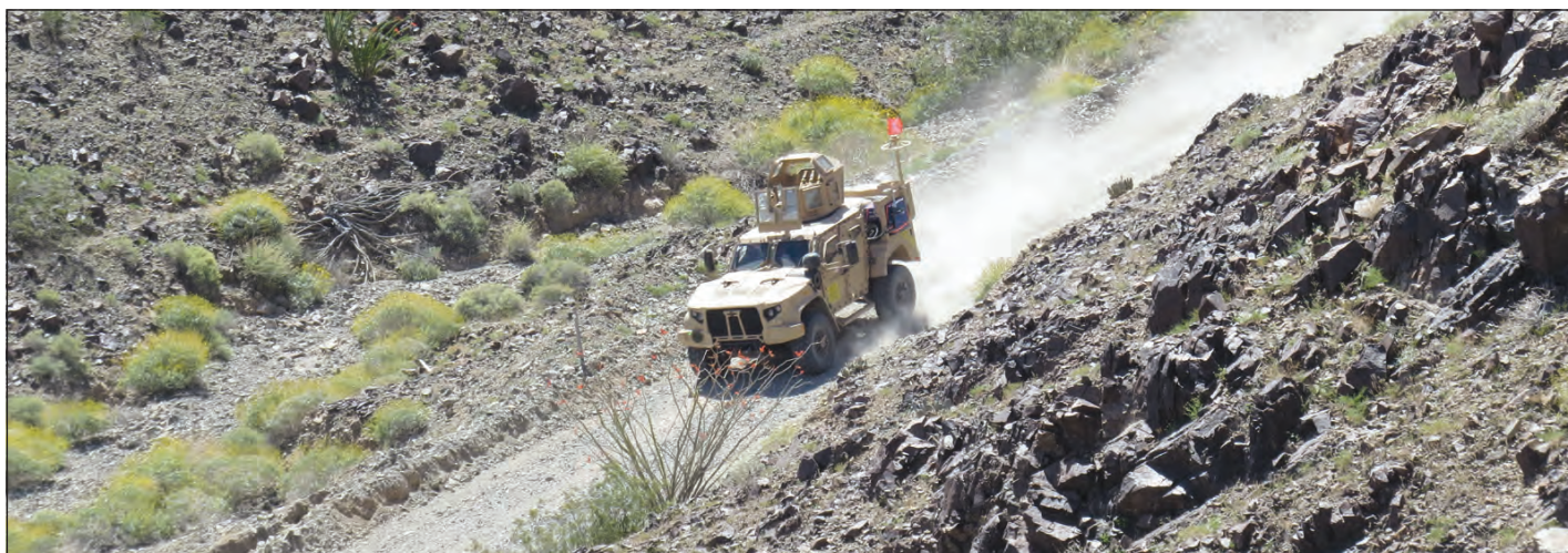
The Joint Lightweight Tactical Vehicle incorporates a long list of upgrades that will make it significantly more advanced than the current tactical vehicle fleet. It sports a height-adjustable, off-road racing inspired suspension, allowing the high-profile vehicle to be lowered to within inches of the ground to facilitate boarding and stowage on ships. Other notable improvements include embedded diagnostics, smart display units, and an automatic fire extinguishing system in the event the vehicle is subject to an improvised explosive device. (US Army Photo)
