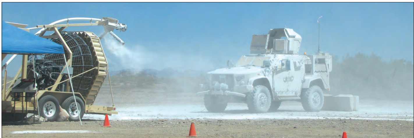
The ravages of sand and dust are daily realities that must be planned for in places where American Soldiers are currently deployed. Though YPG has both in abundance, test items are subjected to controlled and sustained exposure of blowing silica powder or sand for six hours at a stretch, and are often put through their paces on the test range as soon as the punishing sand and dust blasting is completed.
