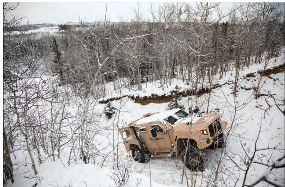
In addition to running the vehicles across 36,500 miles of paved, secondary, trails and cross-country roads at YTC, YPG testers are testing everything from the overhead gunner’s protection kit to vehicle’s active suspension system. The JLTV has also undergone testing at Cold Regions Test Center, as seen here. (US Army photos)
