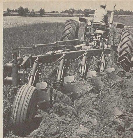
HYDRAULIC self-reset became maximize speed and acreage covered on this Massey-Ferguson 880 moldboard plow. Various bottoms are available for different soil types.
