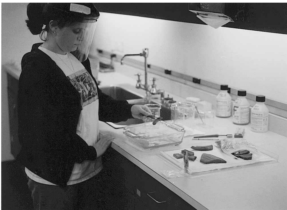
Figure 9. The full face shield protection for the person performing the treatment and the use of forceps to gently lower the sherds into the hydrochloric acid.
