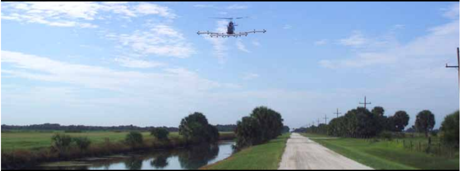
The open prairie-type conditions at Avon Park Formerly Used Defense Site are ideal for using the helicopter magnetometer to search for munitions debris at the site. Flying about 30 to 40 mph, the helicopter detects ferrous metallic debris. (PHOTO COURTESY CORPS CONTRACTOR, ZAPATA)
