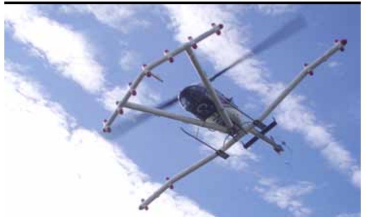
The helicopter magnetometer detects magnetic anomalies on the ground or in shallow subsurfaces. The device flies six feet above ground at speeds of 30 to 40 mph. (PHOTO COURTESY CORPS CONTRACTOR, ZAPATA)
