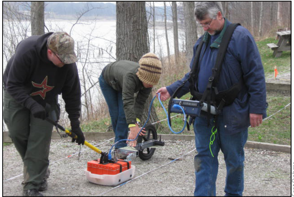
Carl Carlson-Drexler (left), Dominique Cordy and Mike Hargrave use ground penetrating radar on a camp pad in Kil-So-Quah Campground at J. Edward Roush Lake in Indiana.
