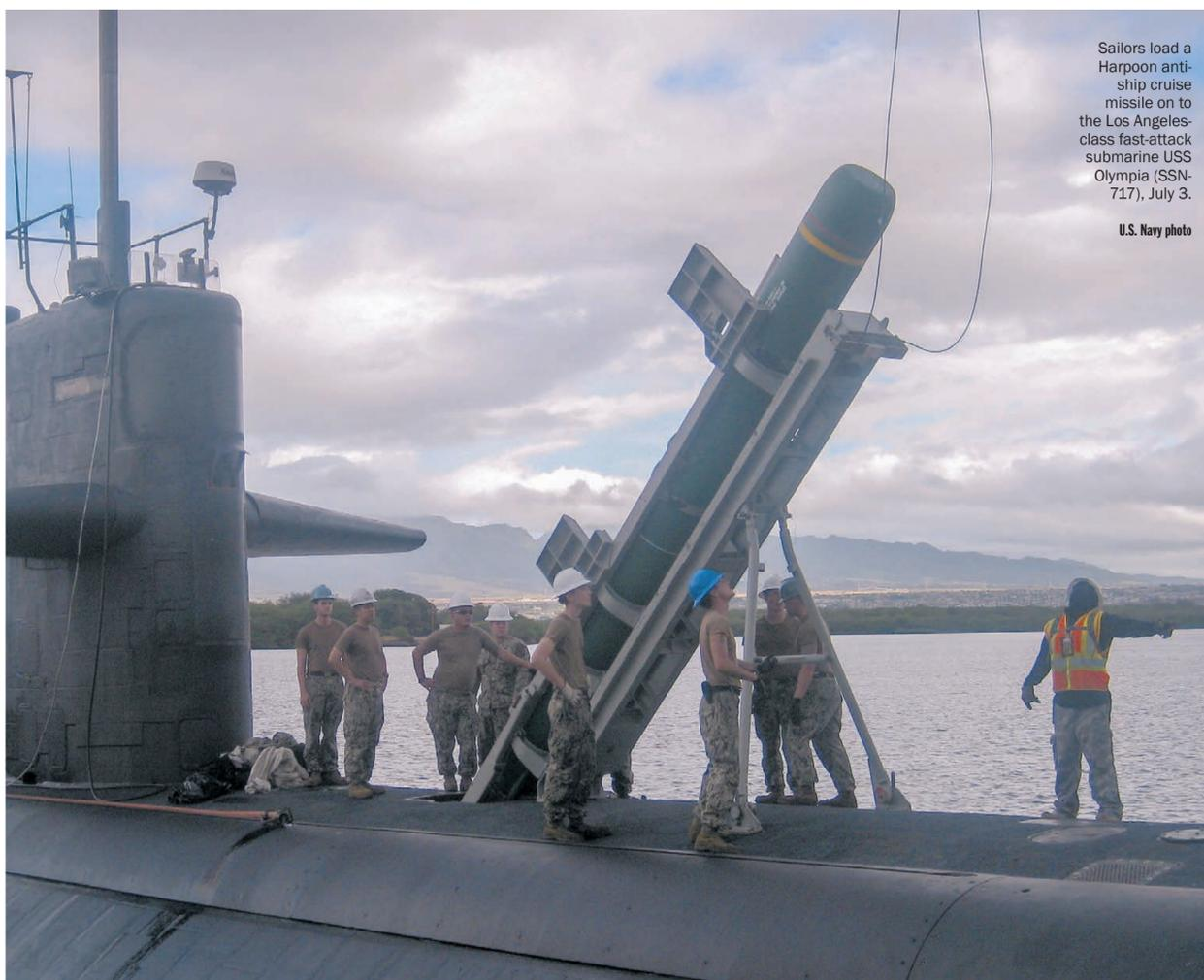
Sailors load a Harpoon anti-ship cruise missile on to the Los Angeles-class fast-attack submarine USS Olympia (SSN-717), July 3.
