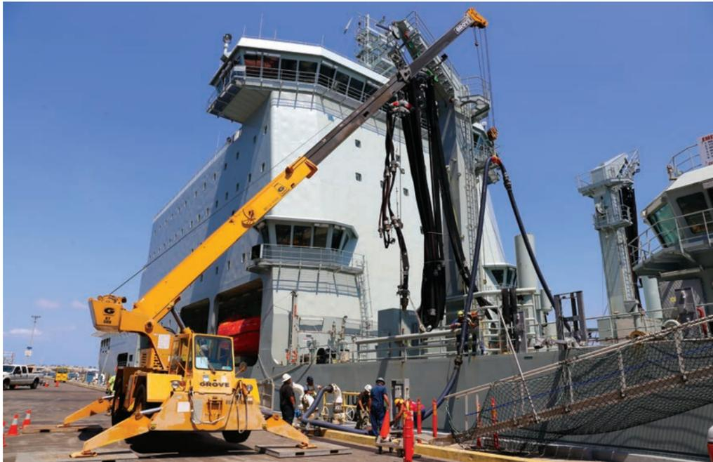
NAVSUP FLC Pearl Harbor personnel hoist fuel hoses to rig to a coalition oiler in preparation for a fuel transfer during RIMPAC 2018.
