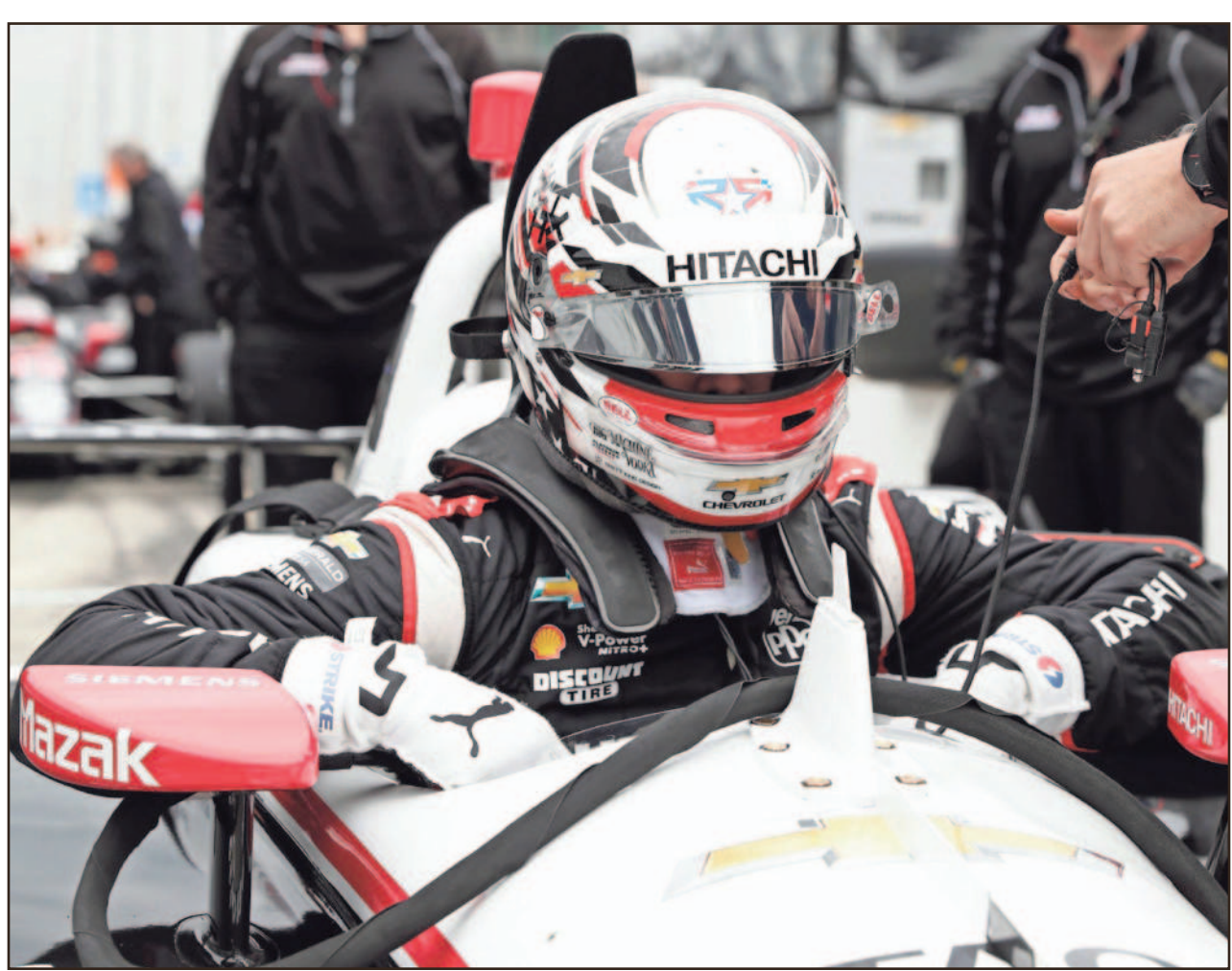
The Advanced Frontal Protection device is shown in front of IndyCar driver Josef Newgarden during testing at the Indianapolis Motor Speedway, Wednesday. The device is supposed to act as a debris deflector to reduce head injuries during wrecks.
