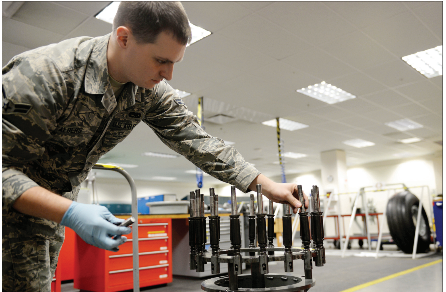
Airman 1st Class Clark Albers, C-17 Globemaster III crew chief and aerospace maintenance journeyman, sets up lugs using a wheel and tire assembly fixture in the Wheel and Tire Shop at Joint Base Elmendorf-Richardson Dec. 18. (U.S. Air Force photo/Airman 1st Class Crystal A. Jenkins)
