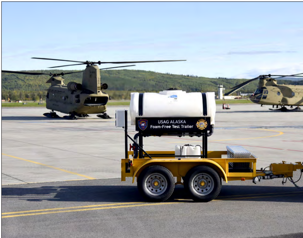
The foam-free test trailer will be used to ensure that fire trucks and pumpers designed to respond to aviation fuel fires are functioning at their peak, while being protective of the environment. (Photo by Brian Schlumbohm, USAG Alaska Fort Wainwright Public Affairs)
