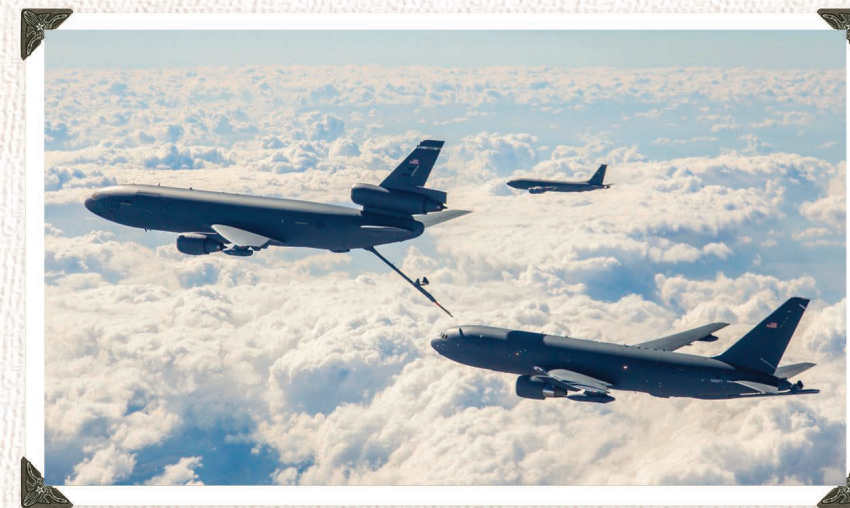
On 19 October 2015, a Boeing KC-46A, lower right, undergoes tests of aircraft acceleration and vibration exposure while flying in receiver formation at various speeds and altitudes behind either the KC-10 Extender or the KC-135 Stratotanker. Testing for this phase was coordinated from Edwards Air Force Base, California. Delivery of operational KC-46 aircraft is scheduled for Fiscal Year 2018. (U.S. Air Force Photo by Christopher Okula).
