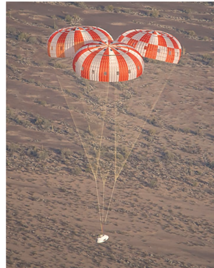
PTV under three good Capsule Parachute Assembly System (CPAS) main parachutes. (Courtesy Photo).
