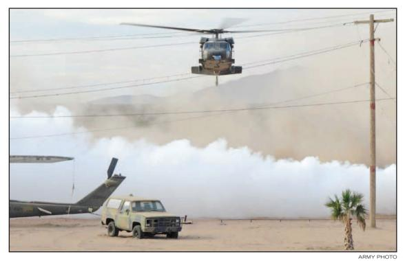
Experimental test pilots participate in degraded visual environment flight testing.
