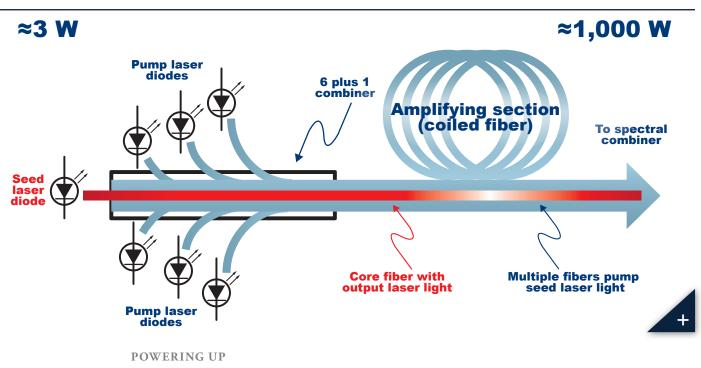
Combined-fiber lasers show great potential for use in laser weapon systems on tactical and combat platforms because they convert electrical power efficiently to power on target. However, today's fiber laser modules are limited to a little over a kilowatt. So, to reach higher power levels, the individual fiber laser modules must be combined into one beam. This diagram shows how the combination process works. (SOURCE: SMDC/ARSTRAT)
