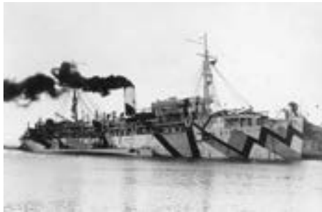
Originally built as a freight/passenger ship, the Beaver had a Newport News vertical triple expansion reciprocating engine that was fed by six Scotch boilers, that produced 190psi of saturated steam.
