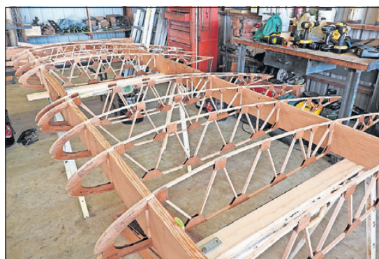
LEFT: The wood structures of the wings are being built for the Stearman. RIGHT: Kal Kimball, left, and his dad Kevin pose with the family flying machine. Three generations of Kimballs have flown this plane.
