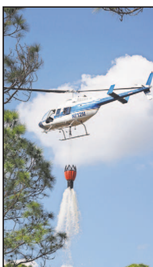
A helicopter demonstrates the use of a Bambi Bucket at last year’s Sarasota County Fire Fest. Bambi Buckets are used to fight wildfires.
