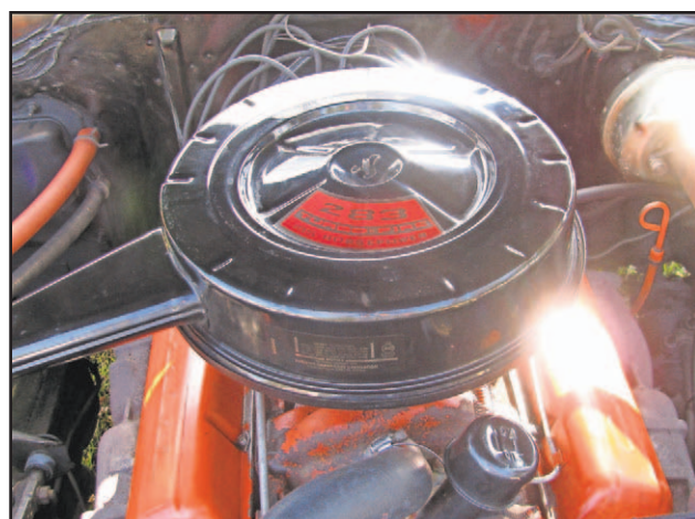
Basic V8 283 Turbo Fire, 195 HP engine of the '65 Chevy SS
