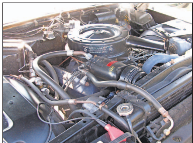
1965 Cadillac DeVille V8, 429 cubic inch, 340 HP engine
