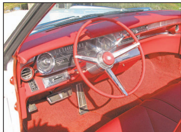
Dash and instrument panel; parking brake lower left of dash of the 1965 Cadillac
