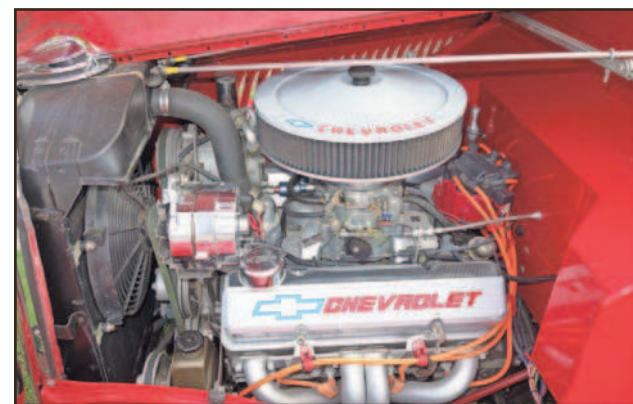
Very powerful Chevrolet engine showing 750 Edelbrock carburetor and headers
