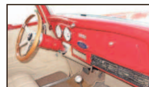
Dash showing instrument panel, A/C ducts, shifter lever and deluxe wood steering wheel
