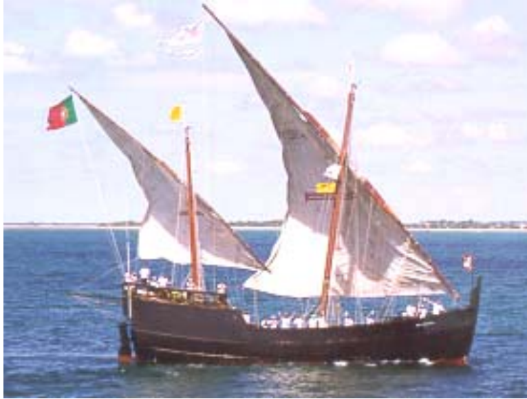
Figure 6.5: A caravel is a small highly maneuverable ship with two or three masts.
