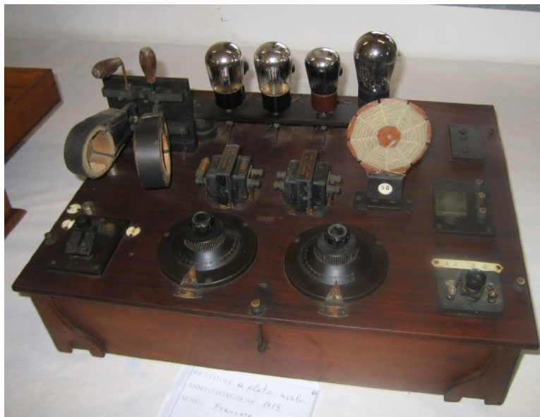
Figure 6.25: An early radio receiver. The four silvery cylindrical objects along the back of the receiver are vacuum tubes.
