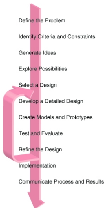
Figure 4.5: A spiral design process. Changes are made in the design, and then the improved design is evaluated.
