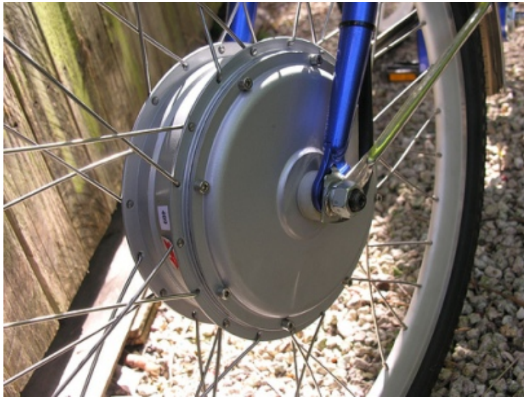
Figure 4.11: This bicycle hub contains an electric motor that moves the bicycle.
