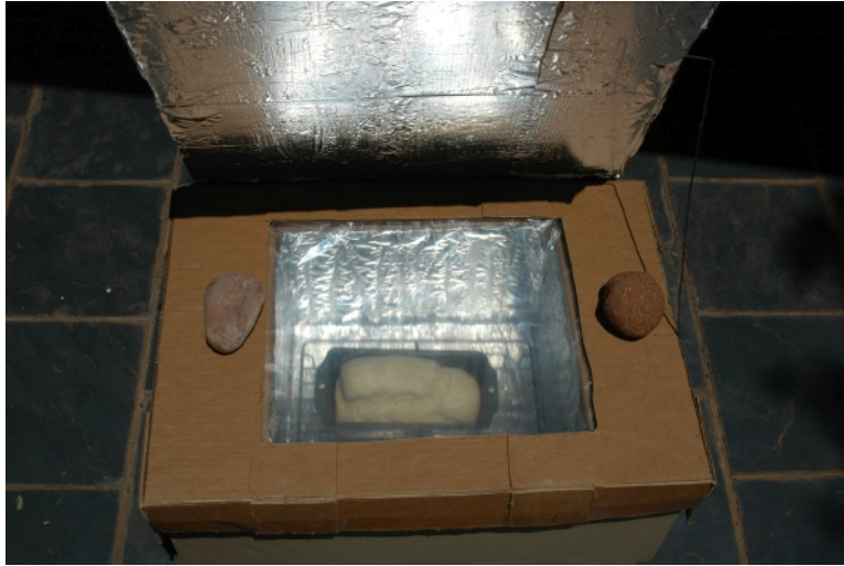
Figure 4.19: A simple solar oven made out of a cardboard box, foil, and clear plastic.
