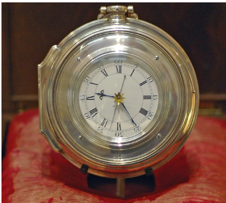
Figure 6.11: H5, the last in a series of maritime chronometers invented by John Harrison to measure time accurately enough to compute longitude.
