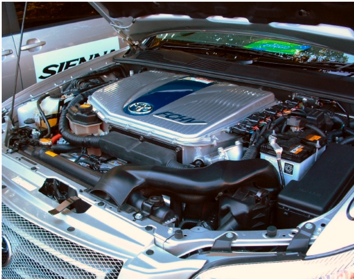
Figure 4.10: The Toyota Fuel Cell Hybrid Vehicle is powered by a fuel cell that generates electricity from hydrogen and oxygen. The fuel cell is still experimental technology that is currently extremely expensive, but shows promise for the future.
