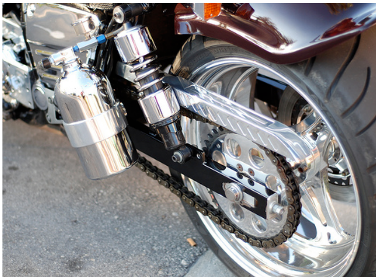
Figure 4.12: This chain drive transmits power from the motorcycle engine to its rear wheel.
