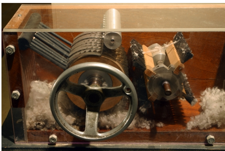
Figure 6.13: Internal workings of the original cotton gin developed by Eli Whitney.
