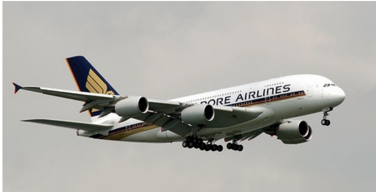
Figure 2.5: The Airbus A380 is the largest commercial jetliner in the world. It can carry up to 850 passengers in two passenger decks in the fuselage.
