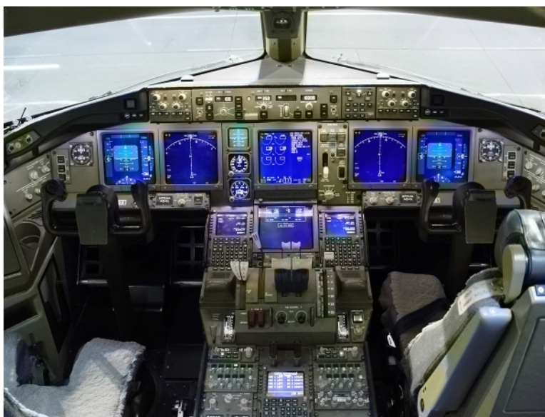
Figure 6.31: The cockpit of the Boeing 777. Note that most flight information is displayed on several computer operated displays.
