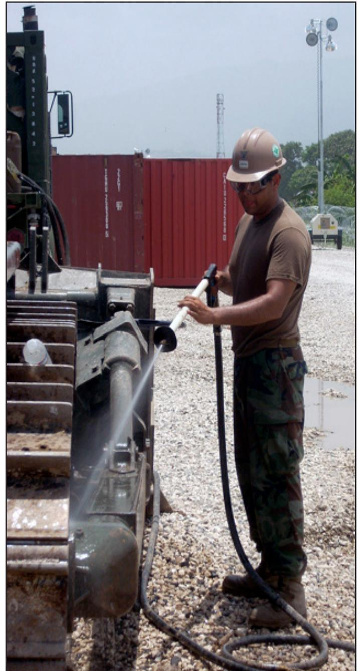
A service member conducts safety awareness by wearing goggles while washing off a vehicle. He also wears a helmet and does not horseplay while working with dangerous equipment. (Photo courtesy of U.S. Army)
